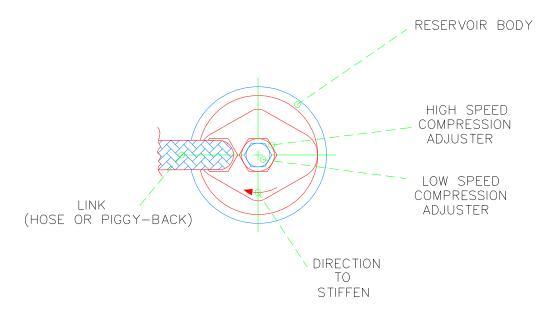
High speed compression control (11mm A/F Spanner)
